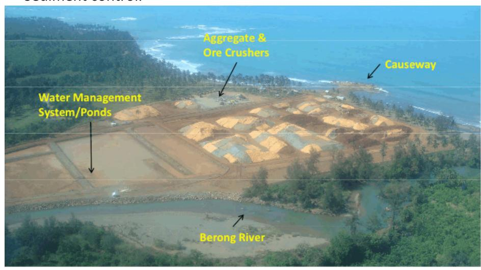
**Sediment Control & Ore Drying;** All mine run off directed to these ponds. Note bottom right – rice farmers use discharge for wet rice, position contra NGO's and Environmentalists.
